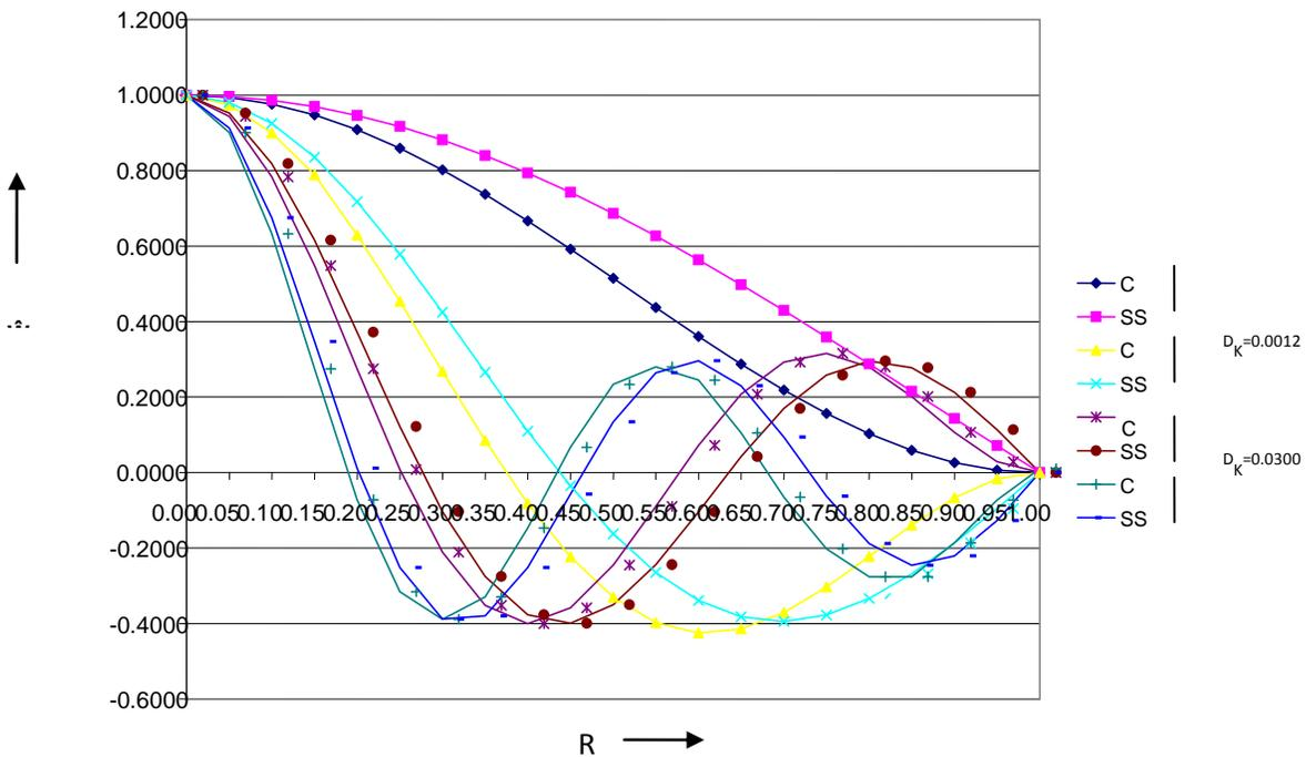
**Fig. 6: Moment Parameters 'M' At Diferrent Point's Of An Circular Damped Plate For The First Four Modes Of Vibrations Under The Parabolically Temperature Field**
