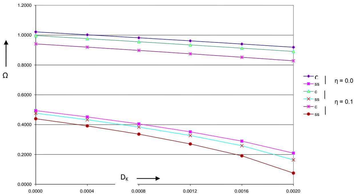
**Fig. 2: Variation Of Frequency Parameter ' $\Omega$ ' With Damping Parameter ' $D_k$ ' For A Circular Plate Corresponding To Second Mode Of Vibration Under The Parabolic Thermal Gradient 'H'.**
