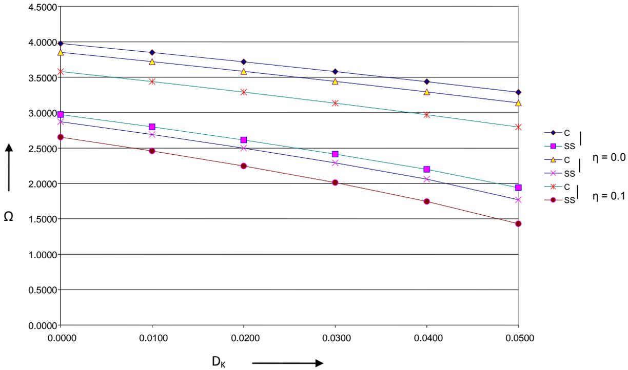
**Fig. 3: Effect Of Parabolic Thermal Gradient 'H' On The Frequency Parameter ' $\Omega$ ' Of A Circular Damped Plate Corresponding To First Mode Of Vibrations.**
