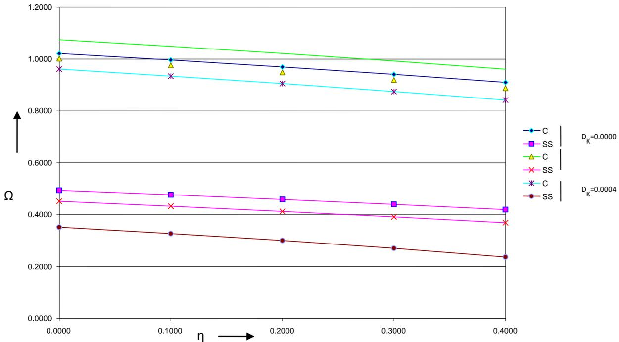
**Fig. 4: Effect Of Parabolic Thermal Gradient 'H' On The Frequency Parameter 'Ω' Of A Circular Damped Plate Corresponding To Second Mode Of Vibrations.**
